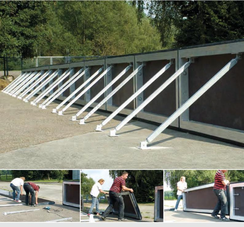
The assembling of one segment requires about 5 minutes. 30 running meters can easily be put together in one hour by two people.
